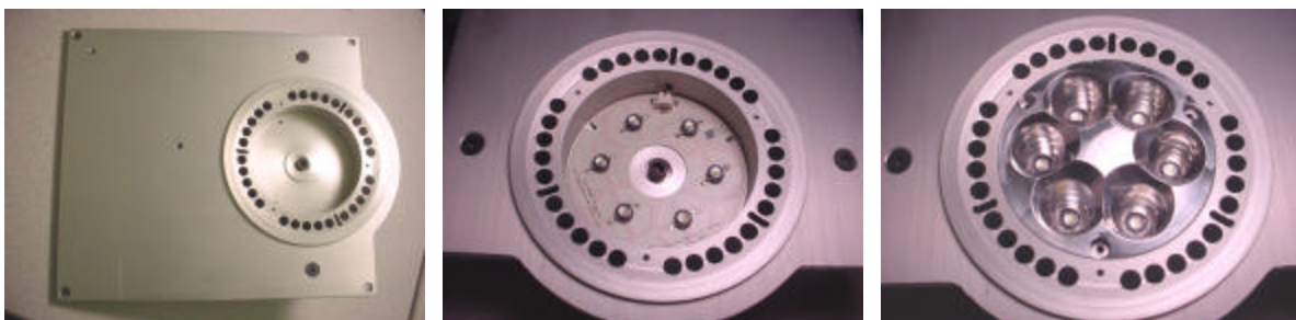
Figure 3. Top view of reflector (left), LED ring with six 3-W Luxeon emitters (center), and bottom view of reflector.
