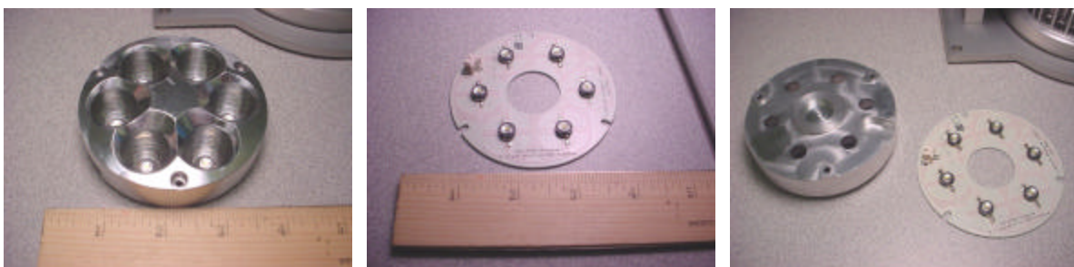
Figure 3. Top view of reflector (left), LED ring with six 3-W Luxeon emitters (center), and bottom view of reflector.
