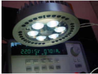
Figure 5. Bottom view of the heatsink and reflector with LEDs turned on during temperature measurement.
