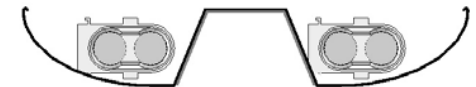
Dual lamps and a perforated fixture provide glare-free direct and indirect light.
